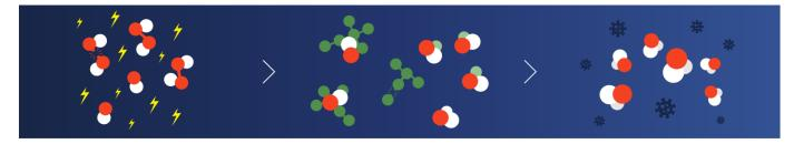
1. UV rays transform hydrogen peroxide into highly reactive hydroxyl radicals.
